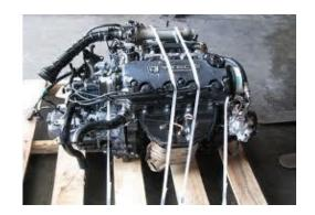
Plastic band strapped engine. 4 plastic straps done by machine and tight. Engine sits flat on pallet, no tyre needed. Ideally should be sat on rags/mat, but not needed as engine is drained, and is very clean. Straps could benefit from protection, but if bands touch smooth areas then are ok.
